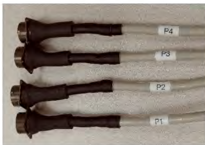
Figure 3 – Cannon to Extension Cables
