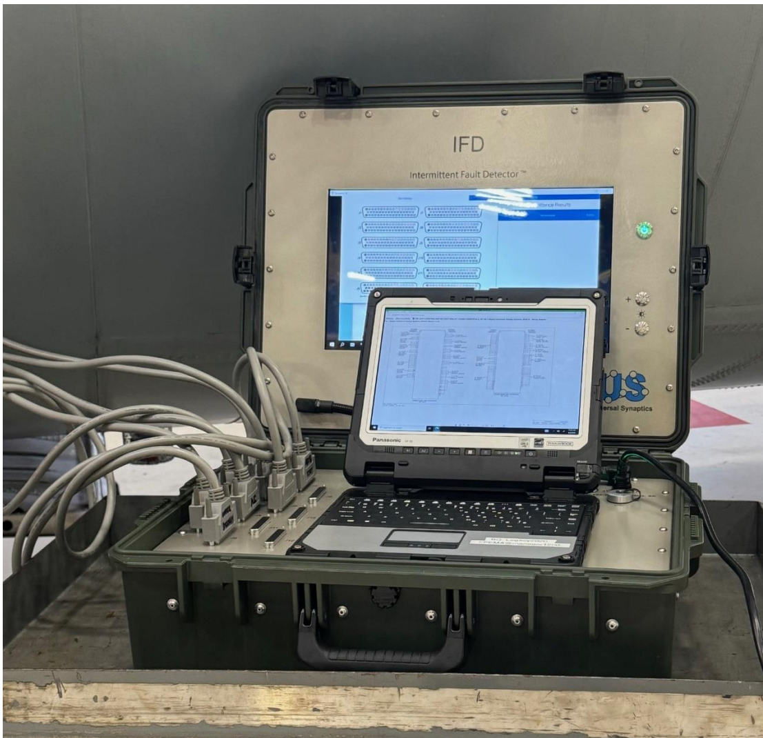
PIFD connected to the C-130 EIDS wiring harnesses.
