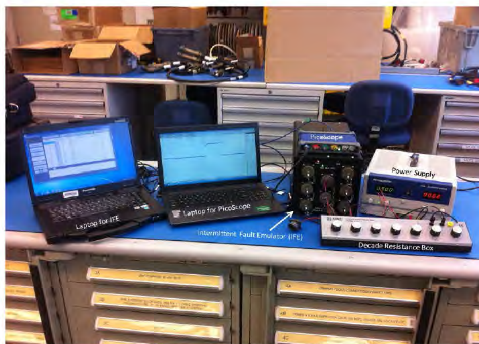
FIGURE B-1. IFE waveform test setup .
