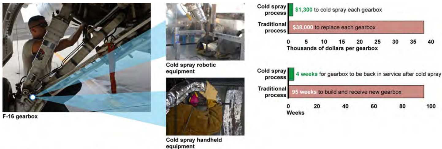
Figure 7: Benefits of Cold Spray Technology for the F-16 Gearbox
