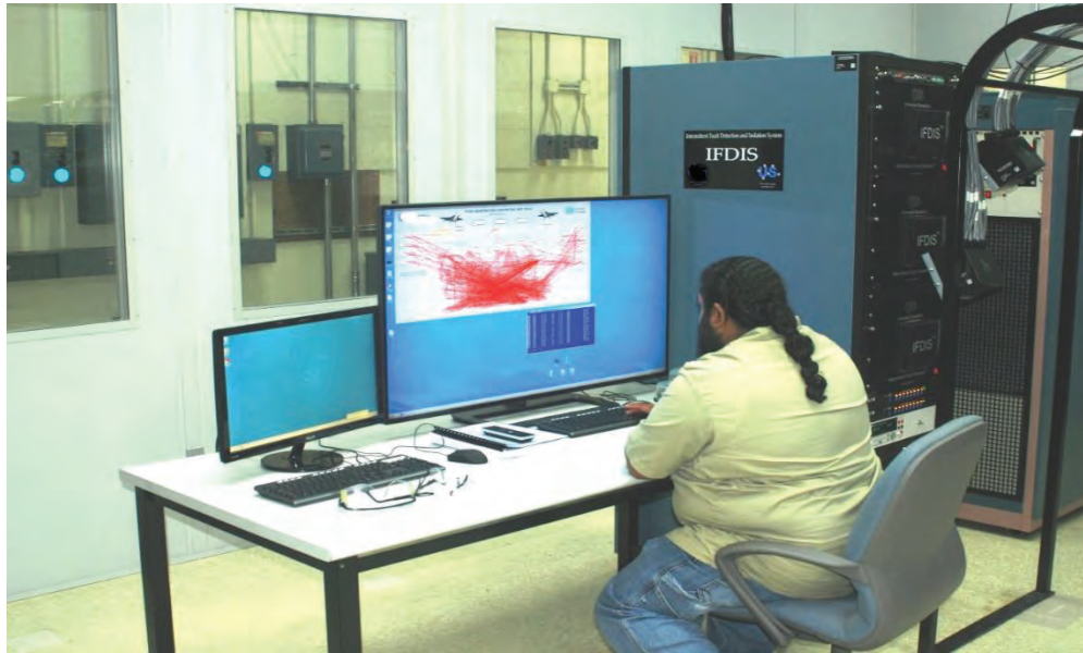
Figure 4. Technician operates the IFDIS to test the GCU chassis of an F/A-18. The IFDIS not only checks the connection points in the GCU harness for intermittent shorts or opens, but also has the capability to simulate the flight stresses and conditions which F/A-18 aircraft are exposed. (U.S. Navy Photo)
