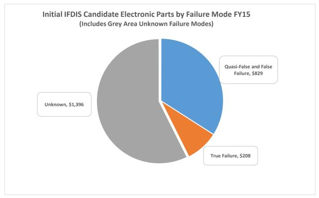
Using FY15 data and isolating potential LRU, WRA type objects and NIINs, the failure recipe tagged \$829 million costs as quasi-false and false failures and \$208 million in cost as true failures.
