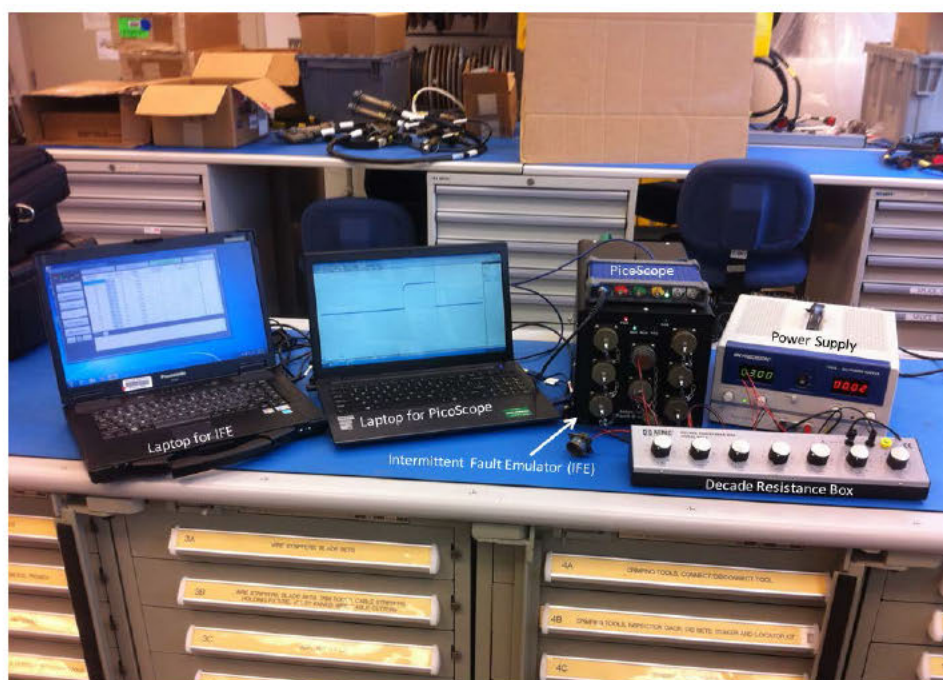
FIGURE B-1. IFE waveform test setup .
