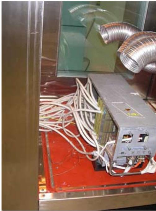
*Outside Figure 1 - Intermittent Fault Detection and Isolation System (IFDIS) from TQS/ Universal Synaptics, Ogden, Utah. IFDIS continuously monitors all 700+ circuit interconnections within this "black box" that is being temperature and random vibration stressed for screening. IFDIS is watching for any otherwise undetectable low-level nano intermittencies.*
